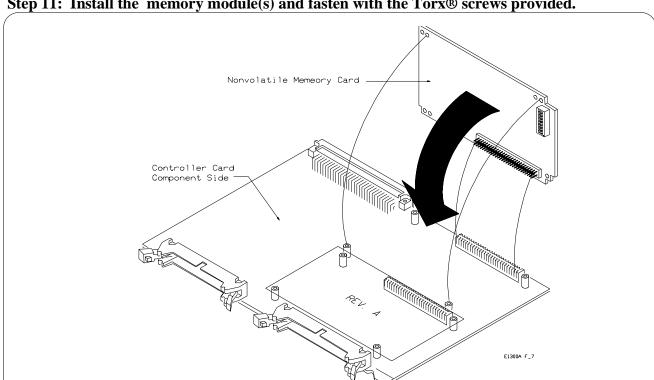
Step 11: Install the memory module(s) and fasten with the Torx® screws provided.
