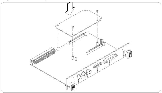
Step 5: (Optional) Install second memory module and fasten with four Torx® screws.
