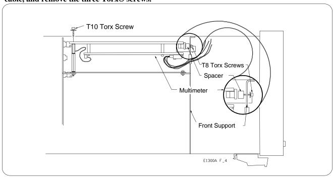
**Step 7: Remove the multimeter.**
