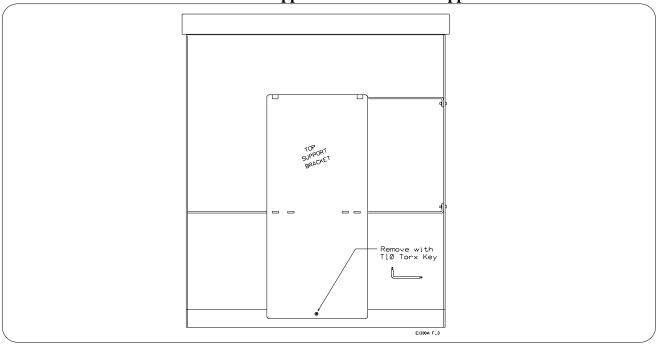
Step 6: If you have an internal Agilent E1326 5 1/2 Digit Multimeter, disconnect the BNC cable, and remove the three Torx® screws.
